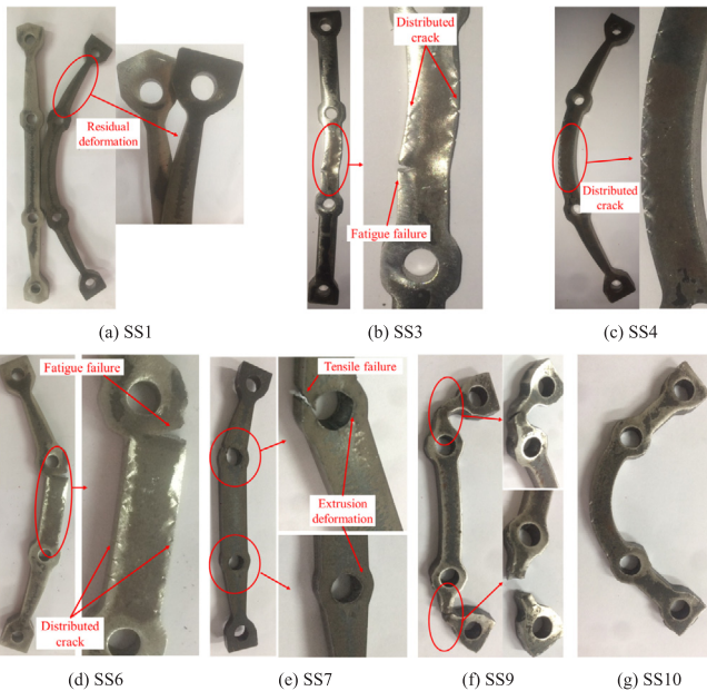
Fig. 6. Deformation and failure conditions.
