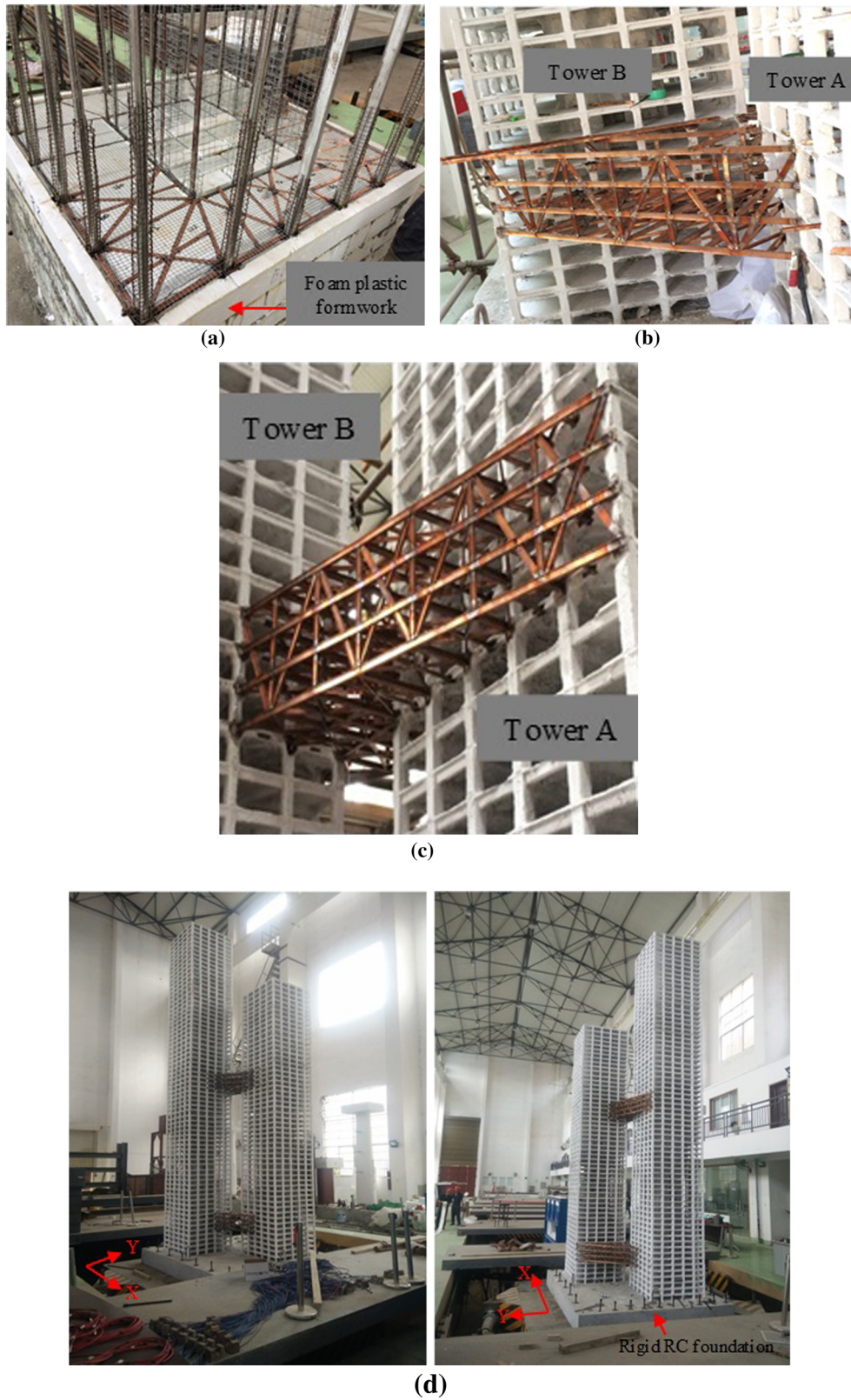
FIGURE 6 Construction of the test model structure. (a) Structural member manufacture. (b) Connecting truss of fifth to eighth floor. (c) Connecting truss of 33rd–36th floor. (d) The test model
