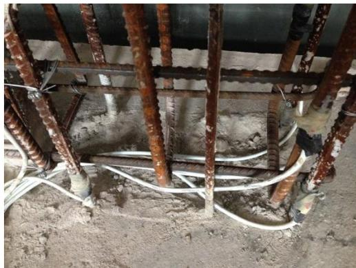
(b) 后浇区钢筋应变测点布置
