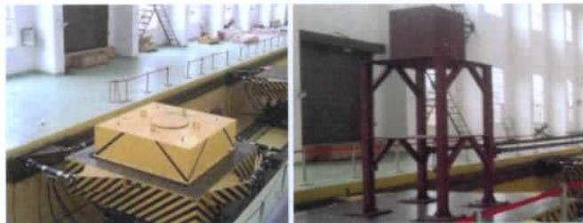
(a) 18.5t 的惯性试件 (b) 弹性试件 (a) Inertia specimen of 18.5 ton (b) Elastic specimen
