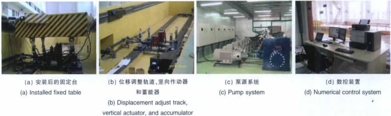
图 2 中南大学地震模拟振动台 Fig. 2 Earthquake simulation shaking table located at Central South University
